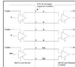
For encoder connections of distances greater than 22m refer to factory.
