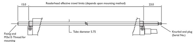
The encoder reader-head is to be installed within 50µm (0.002 in.) end-to-end relative to the axis of the scale in both horizontal and vertical planes
